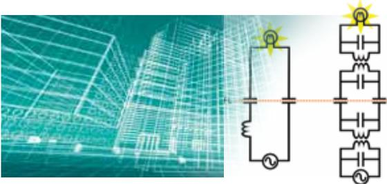
Architectural firm Takenaka Corporation develops wireless power supply systems that are embedded in the walls and floors of buildings. In designing the circuit for this system, the company coupled several ANSYS tools to determine capacitance between electrodes, to create the inductor design, and to analyze the electromagnetic radiation characteristic.
