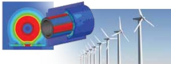
One rising trend in wind turbine generation is permanent magnet generators, offering higher efficiency and design flexibility. Indar Electric used our tools to reach the ambitious target of 97.7 percent level efficiency at rated load in converting mechanical to electrical energy.
