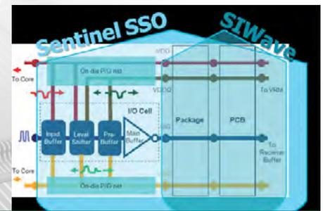
**SIwave:** LSI Corporation used ANSYS Chip Signal Model and ANSYS SIwave to show that voltage swings on the signal network of a DDR parallel interface circuit were coupling to the power supply of the PLL, resulting in phase error between the PLL reference clock and output clock.
